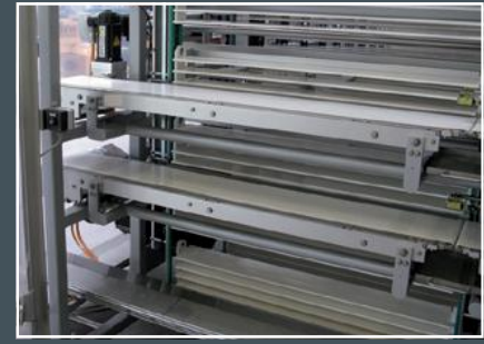
1 Level change: PFR input and output can be located on different floor levels 2 FSU: Integrated high-speed loading with waste rejection 3 Multiple output: To feed multiple packaging legs
