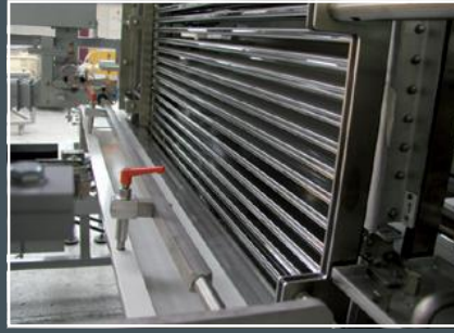
1 Buffer roller chain: Gondolas are accumulated on the roller chain 2 Product output: Product rows are pushed onto the cross feeding conveyor up to the product stop 3 Automatic removal of the gondolas: optional
