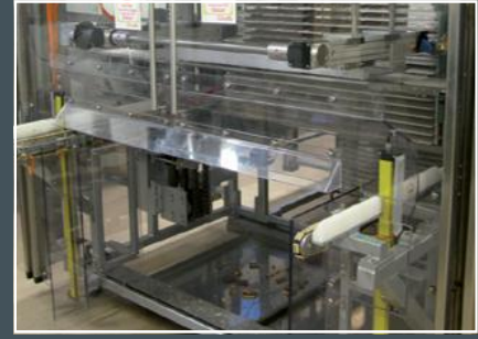
1 Buffer roller chain: Gondolas are accumulated on the roller chain 2 Product output: Product rows are pushed onto the cross feeding conveyor up to the product stop 3 Automatic removal of the gondolas: optional
