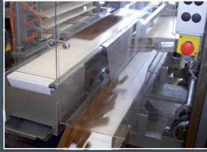
1 Deposit of the rows onto the cross feeding conveyor or the gondola shelf 2 Retraction of the pull nose and discharge of unacceptable rows 3 Feeding of a packaging leg
