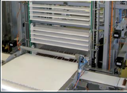
1 Deposit of the rows onto the cross feeding conveyor or the gondola shelf 2 Retraction of the pull nose and discharge of unacceptable rows 3 Feeding of a packaging leg
