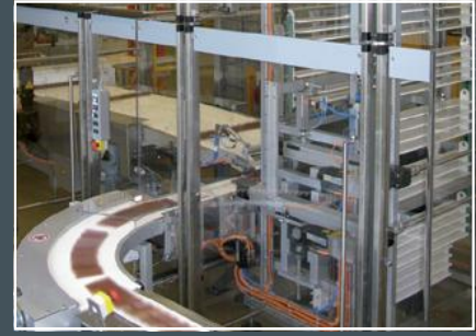
1 Deposit of the rows onto the cross feeding conveyor or the gondola shelf 2 Retraction of the pull nose and discharge of unacceptable rows 3 Feeding of a packaging leg
