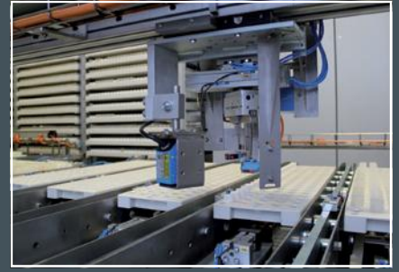
1 Storage Racks with alley for the commissioning robot 2 Commissioning Robot retrieving storage rack 3 Pick and Place Robot
