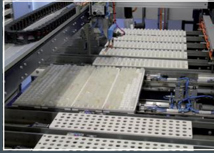
1 Storage Racks with alley for the commissioning robot 2 Commissioning Robot retrieving storage rack 3 Pick and Place Robot
